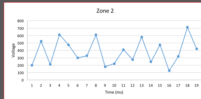
Figure 5 (right). Voltage differences by zone. The further the fish is from the sensor (Zone 3), the higher the voltage valued recorded. At a close proximity (Zone 1), voltage drops to zero and triggers the automatic feeder. Zone areas were measured on the experimental tank in centimeters.
